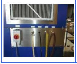
Cooling water inlet: 19mm ID hose. Cooling water outlet: 19mm ID hose. DI water: 10mm ID hose. Drain: 10mm ID hose. Clean air: ø 250mm
