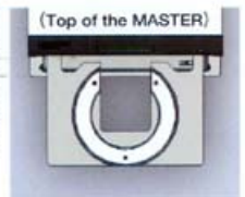
Ⓜ Sufficient space will be provided between the recording surface of a 120mm disc and the top of the tray by removing the adaptor for the 80mm disc.
